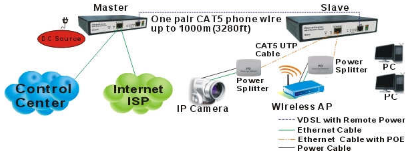
Figure 3: Ethernet Extender Point-to-Point application Ethernet Extender with Remote Power Application
