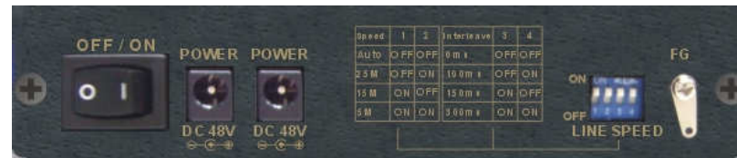
Figure 7: Rear connectors of Ethernet extender for Master and Slave respectively
