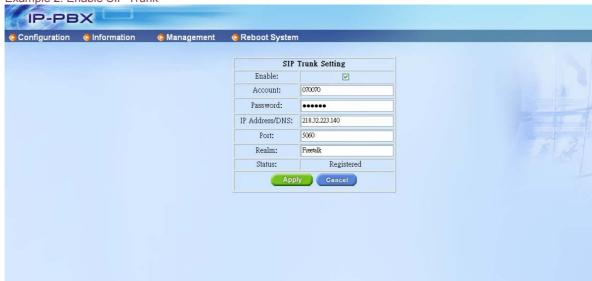
**Enable:** Check to enable this SIP Trunk.
