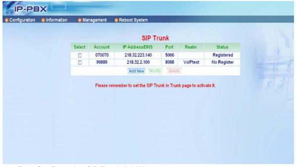
Enter Configuration SIP Trunk-Add New to configure IP PBX-100 register to ITSR ITSP
