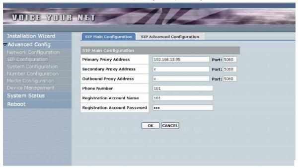
This Example, we have 1 DW register to IP PBX-100 with extension 103 to 106. You can set the SIP Information of 3504 by its COM port or you can also login its WEB interface for configuration as below. Set the 3504 to proxy mode, and also set the Primary Proxy IP Address
