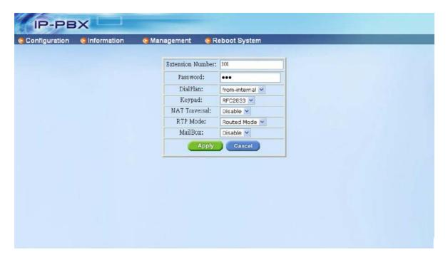
**Extension Number:** Assign the number of Extension. This number is also the register name for device.
