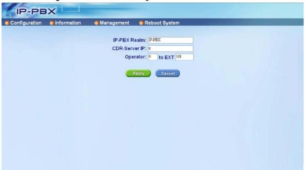
**IP-PBX Realm:** Configure Realm of IP PBX-100. This parameter is essential when there is more than one IP PBX-100, and user wants to have inter-case between IP PBX-100s. Pease refer to SIP Trunk configuration.
