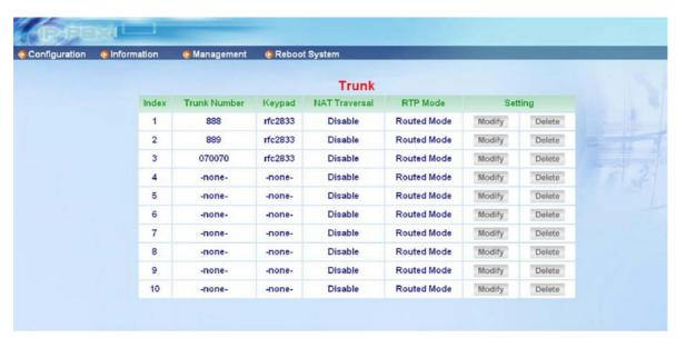
configured Trunk data. Press **Delete** will delete the specified Trunk.
