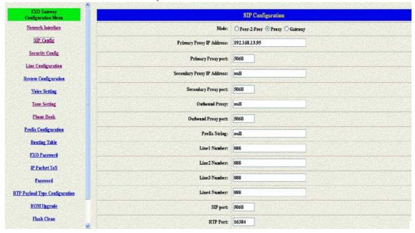
Set Dynamix DW to Proxy Mode, and also set the line number for line1 to line4.
