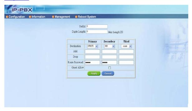
In this example, we set prefix to 0 and there is not limit for digits length (0). The first destination is ITSP and  $2^{nd}$  destination is Dynamix DW (888). And we also set the Routed Password for this prefix route.
