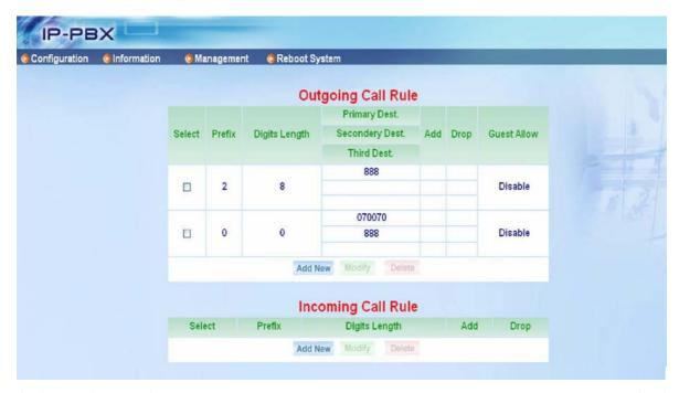
Confirm the Outgoing Cal Rule. Now the Extensions can dial to 0922123123 to reach mobile phone via ITSR If extension called out with prefix number 0, the IP PBX-100 will pay an announcement for route password, after input the correct password, then IP PBX-100 will dial to destination.
