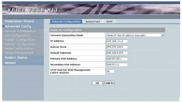
Set IP information for DW. You can set the IP info of DW by its COM port, or you can also login its WEB interface by default IP 10.1.1.3. Go to **Network Interface** page to setup network setting as below. After set the network info, please press OK -\* Commit Data -\* Reboot System. For more information about DW, please go to: http://www.dynamix.ua
