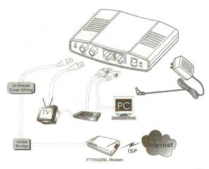
The figure above shows how to connect an xDSL modem to a home coaxial cable network. Follow the same steps to connect any Ethernet device such as a HUB or printer, to a coaxial cable network.
